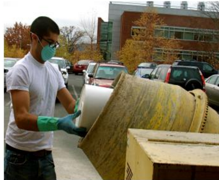
Figure 1 Depiction of Addition of Aggregate to the Mixer
