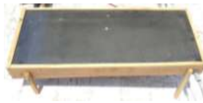
Fig 2: Wire Mesh Solar Air Heater
