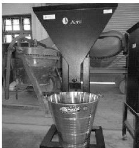
Figure-2: (A) Slump flow test, (B) V-Funnel test, (C) L-Box test
